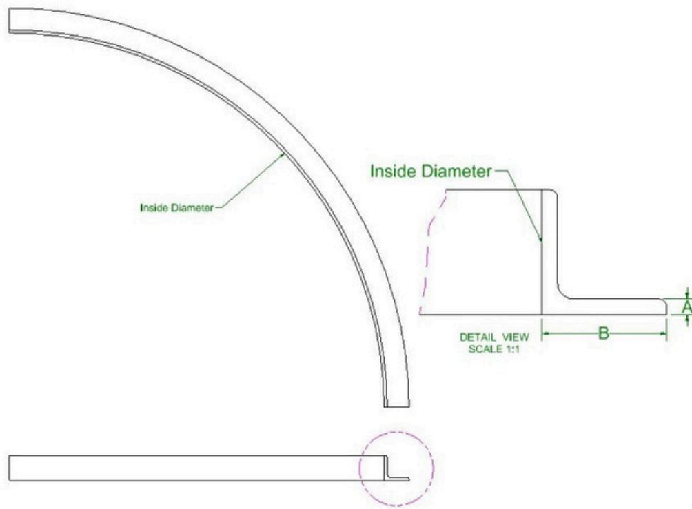
Where A is greater than 1/10th B, and where the inside diameter of the rolled structural is greater than 10X B, rolling is generally possible.
