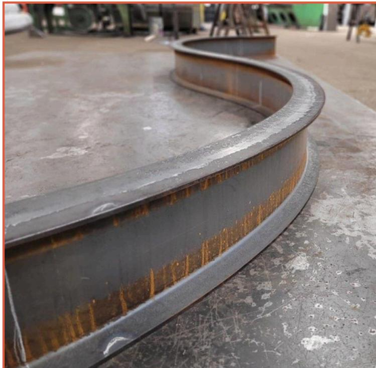
We have had to reject beams as un-formable due to these issues. Please ensure that beams selected for monorails adhere to a high standard of tolerances regarding these areas.
